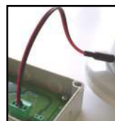
Picture 7 - An example of cable connection between the programmer and a conventional zone module
